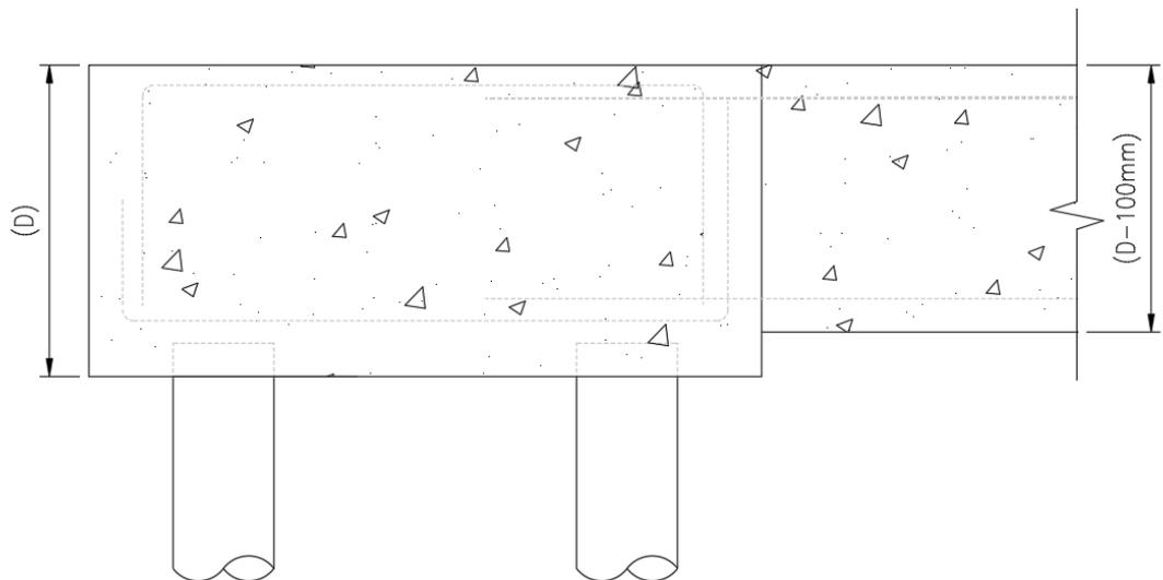
Typical Pilecap-Grout Beam Interface
